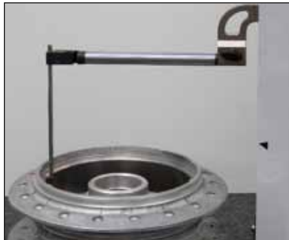
Measurement of a groove using a 90° angled measuring insert holder and an L-shaped insert (TA-IH-105/V.50.5/V-50.3)
