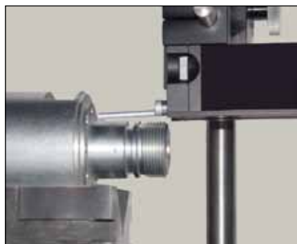
Checking of surface roughness near a shoulder (TA-MS-601)
