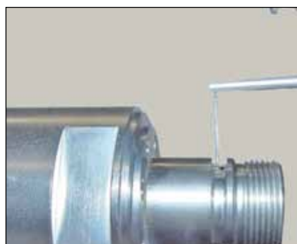
Checking at recessed measuring points (TA-MS-609)
