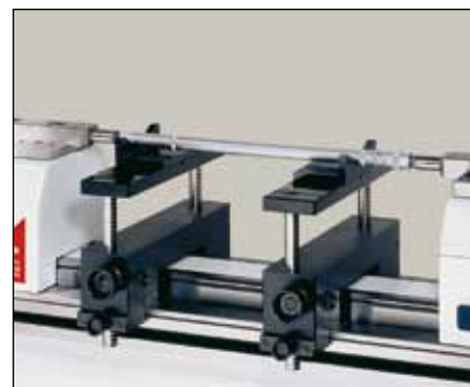
Setting of 2-point internal micrometers (HPA-1/TELMA7/TELMN7.2)
