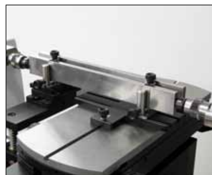
Comparative checking of gauge blocks > 250 mm (TA-SU-307/TEL7/TELMA7)
