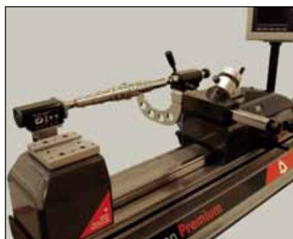
HPA: Measurement of cylindrical parts (TA-MS-303)
