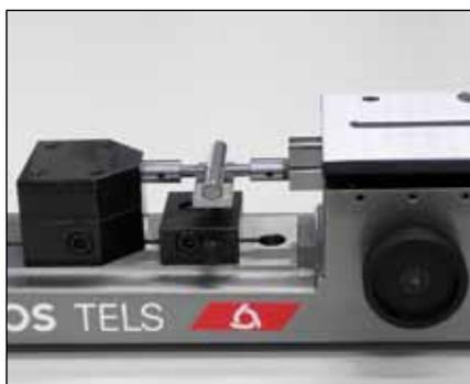
Checking of external diameters
