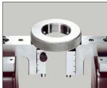
HPA: Checking of thread ring gauges (TEL18)
