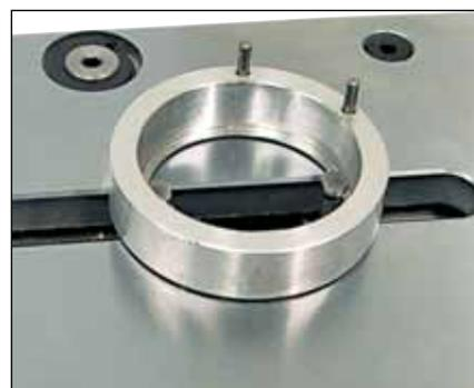
Checking of internal grooves
