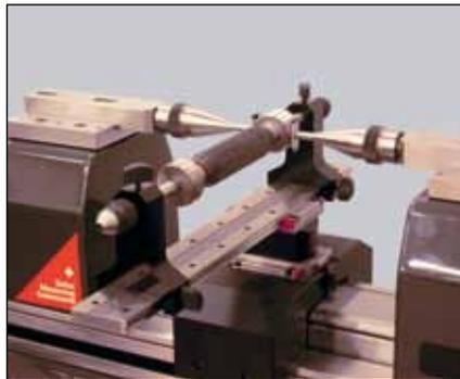
Checking of thread plug gauges (HPA-1/TEL6/3P/0.17-3.2/S6.5/LABC-15)
