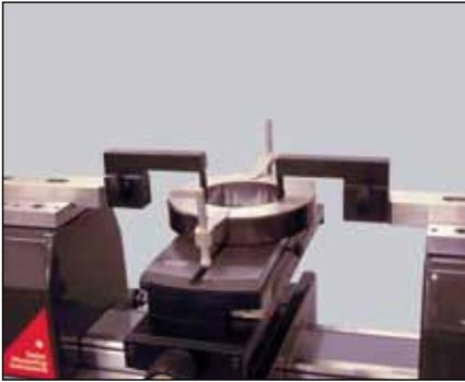
Checking of ring gauges
