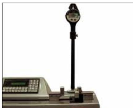
Setting of two-point bore gauges
