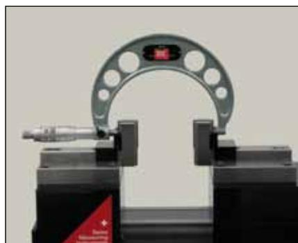
Checking of external micrometers (TEL5/TEL11)
