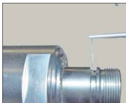
Checking at recessed measuring points (TA-MS-609)
