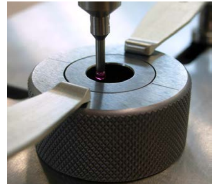
Figure 2 100% automatic calibration of a high precision ring
