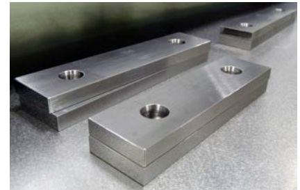
Figure 2 Waiting for calibration: Temperature stabilization of gauge blocks
