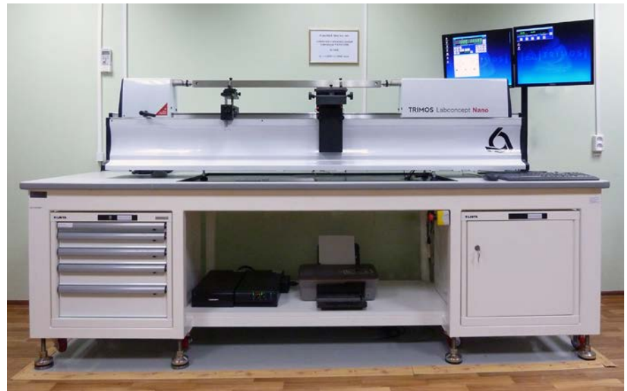
Figure 1 The Labconcept Nano during calibration of a 1000 mm gauge block in the dedicated laboratory for gauge blocks measurements.
