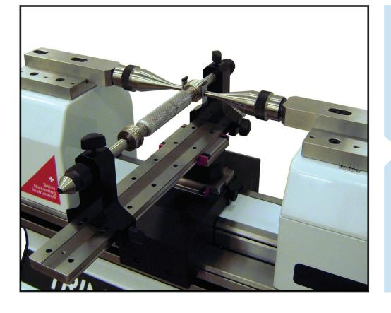
Calibration of plain and thread plug gauges
