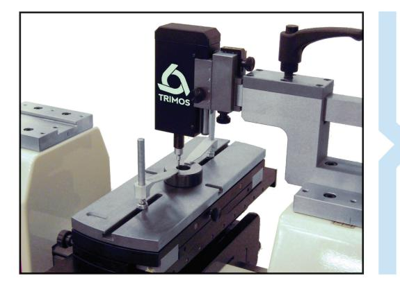
Calibration of plain and thread ring gauges
