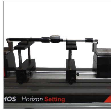
Setting of two points internal and external comparative measuring equipment (TEL5, TELMA7, TELMN7.2)
