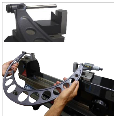
Manually checking of external micrometer (TEL5) (TEL11)
