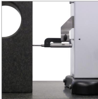
Perpendicularity measurements with electronic probe
