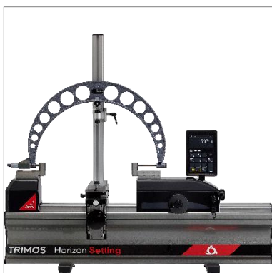
Checking of external micrometer held on a support (TA-SU-313, TA-SU-309, TEL5)
