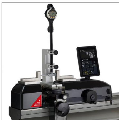
Setting of 2-point bore gauges with holder (TA-SU-313, TA-SU-318, TEL5)
