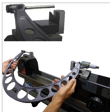
Manually checking of external micrometer (TEL5) (TEL11)
