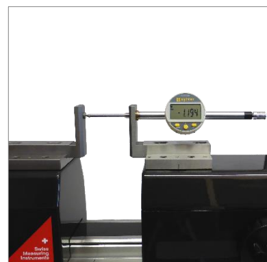
Checking of dial indicator (TEL5CN)
