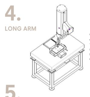
Our long experience in the field of metrology allows us to carry out roughness measurements on complex surfaces that are far apart from each other thanks to a long special arm. Thus, it is possible to carry out 2D roughness measurements according to ISO 4287 on the X or Y axis or in 3D mode.
