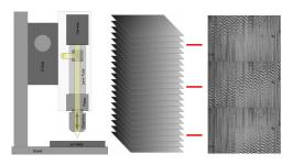
The piezo motor lifts the lens on the z-axis and the camera captures images in equidistant steps.
