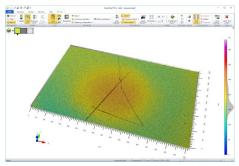
Developed around a graphic interface, the analysis software can work in 2D or 3D. Surface and profile extractions allow the analysis of all roughness parameters in 2D and 3D mode according to current standards.
