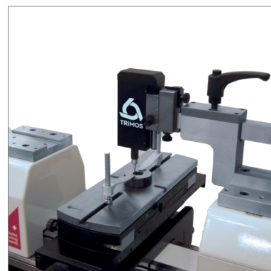
Etalonnage de petites bagues lisses (TA-SU-313, TA-MS-370, TEL76, TA-SU-354)
